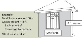
• The grouted stone patterns are packaged assuming a ¾" grout joint. If your grout joint will be different than this, it may be necessary to order more or less product accordingly.
